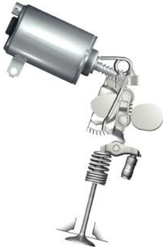
Valvetronic II at maximum valve lift
